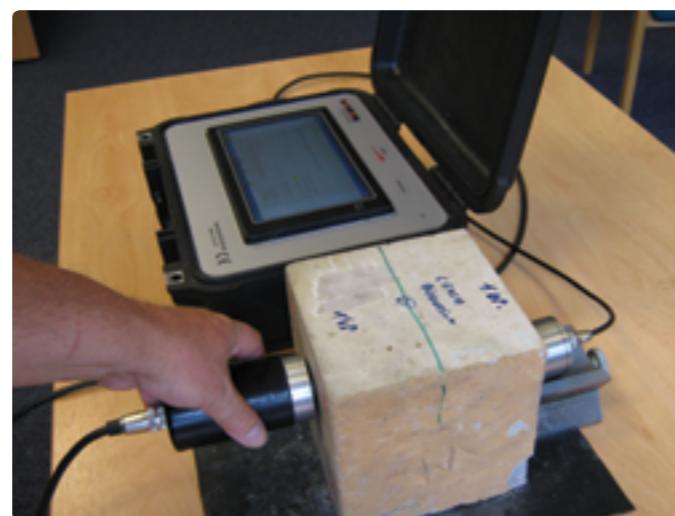
Figure 3: Testing the cube (side view).
